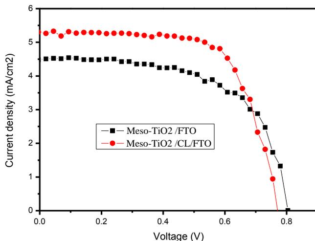
**Figure 3. Current-voltage curves of DSSCs with and without TiO<sub>2</sub> compact layers incorporating with, Co(II/III) electrolyte (0.22 M Co(II) and 0.033 M Co(III), 0.1 M LiTFSI and 0.5M 4-tert-butylpyridine in Acetonitrile). Photo-sensitizer (LEG4).**
